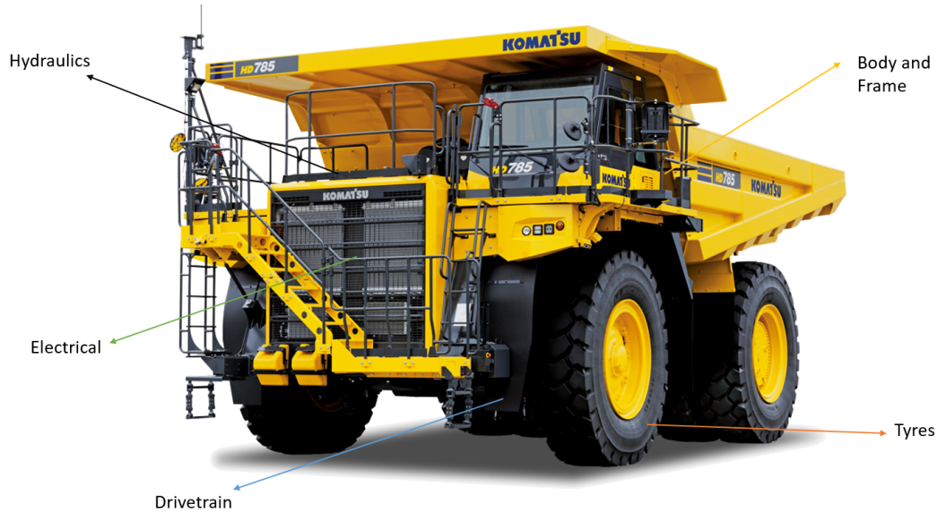
Figure 3.1 Komatsu HD 785 Sub-system Schematic View
